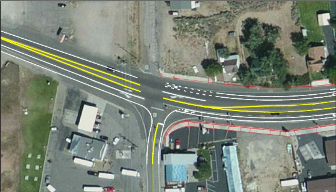
Figure 12. The intersection with Twin Lakes Road will be narrowed to improve safety, sidewalks will be completed, and bike lanes will replace vehicle lanes.
