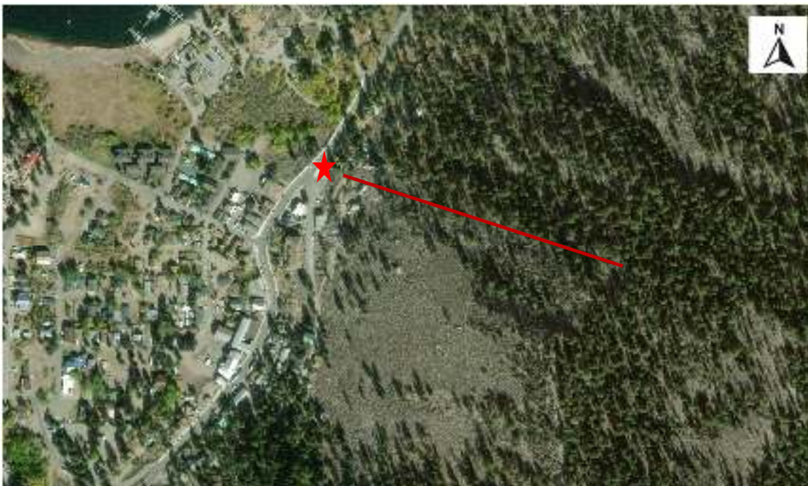
Figure 2. View of Highway 158 and the DeCoster building. The red line indicates the general location of an avalanche path that could reach the DeCoster building and Highway 158.
