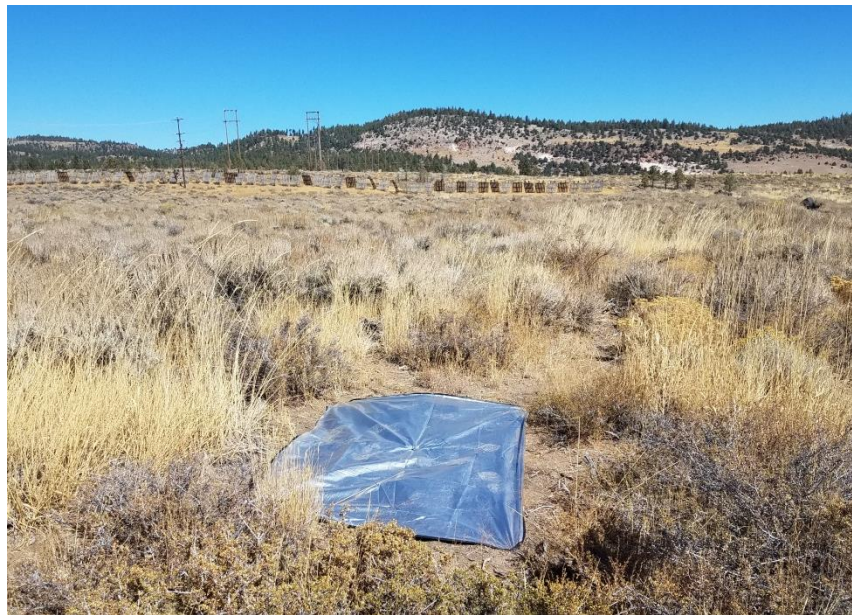
Figure 4. Thermal blanket used to geospatially correct the TIR imagery
