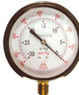
At the fabricator's shop, the testing vacuum in the interstice should be retained for a minimum of 24 hours at -25" Hg. Many tank manufacturers keep the vacuum at this level for 48 hours--my experience says the longer the better.
