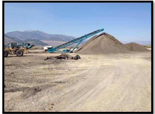
That opportunity became a reality when the County reached an agreement with W. Jaxon Baker Construction out of Redding, CA, who was looking for asphalt feedstock for a paving project in Inyo County. They mobilized crushing equipment to the site and extracted the material from the area where it was disposed over 20 years ago.
