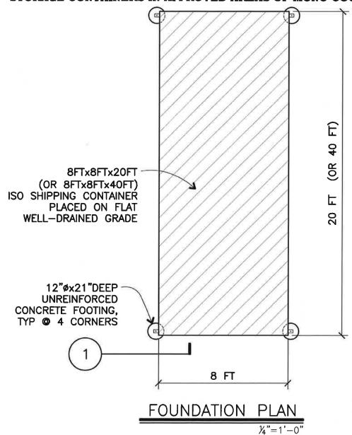
CONCRETE SHALL HAVE A MINIMUM ULTIMATE COMPRESSIVE STRENGTH OF 2500 PSI AT 28 DAYS.
