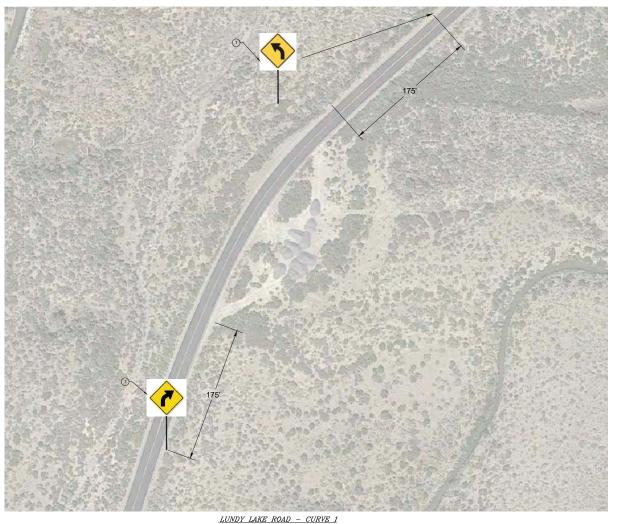
1) INSTALL SINGLE STEEL-POST CURVE WARNING SIGN (W1-2) PER SIGN DETAILS ON SHEET C2..
