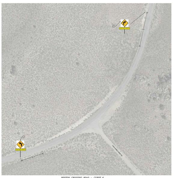
1) INSTALL SINGLE STEEL-POST CURVE WARNING SIGN (WI-10) WITH STREET NAME "CASA DIABLO MINE ROAD" SIGN (WI6-8aP) PER SIGN DETAILS ON SHEET C2.
