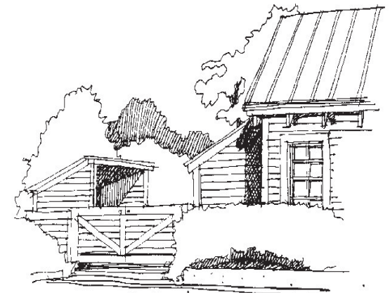
Screening conceals parking and service areas
