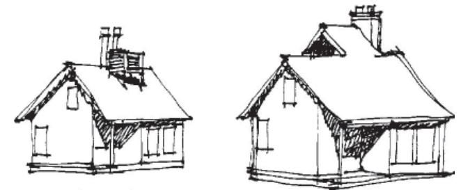
Keep mechanical equipment hidden on roof
