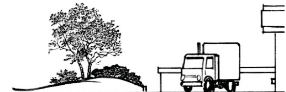
Wall, landscaping and berms screen industrial buildings and storage
